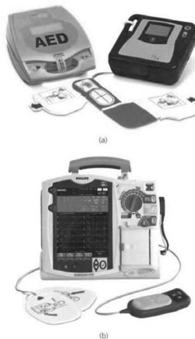
Figure 3. Sophisticated CPR feedback/prompt devices integrated with defibrillators
